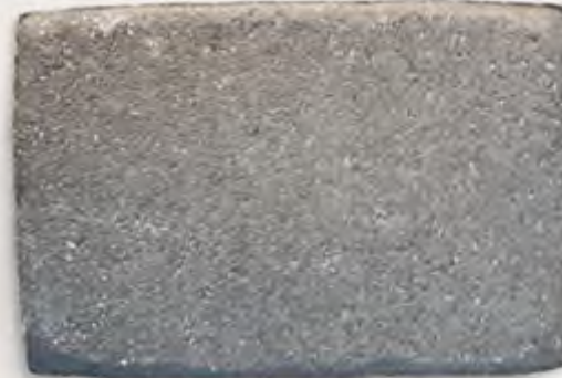
BELGARD COLORGARD PAVER AFTER 15 YEARS OF EXPOSURE
